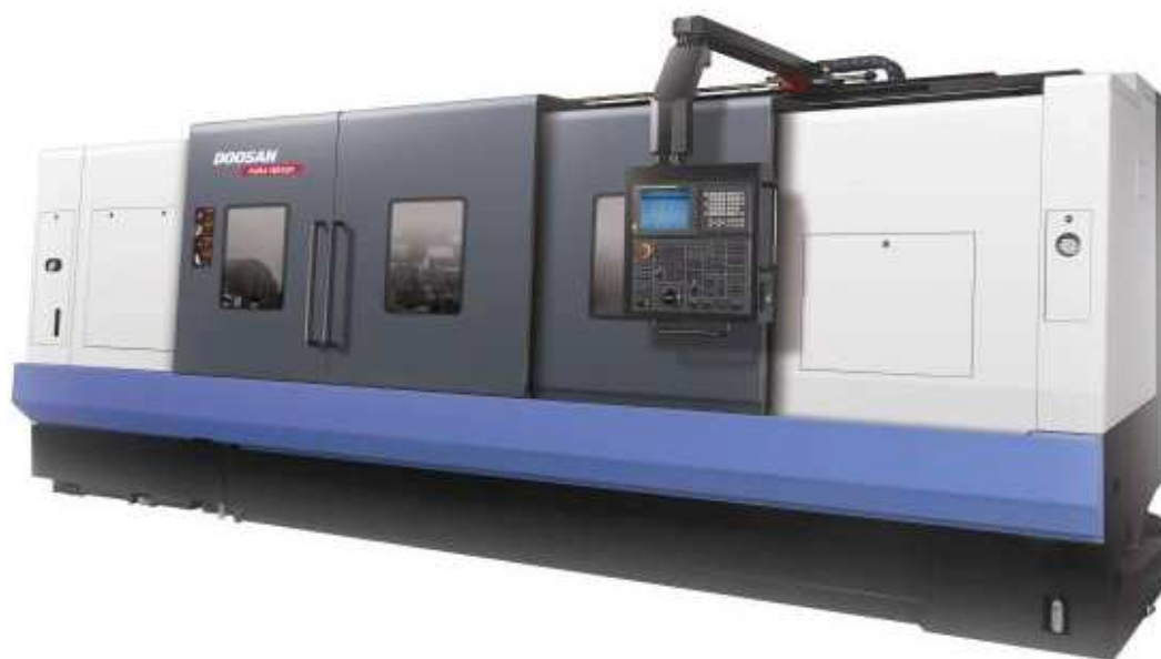
Obr. 4.1 CNC soustruh DOOSAN- PUMA 480 XLM [2].
