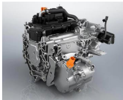
Obr. 6.14 Elektromotor Peugeot e-Expert 100 kW [41]
