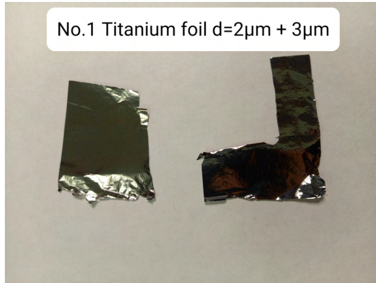
Figure 48 | Nonirradiated titanium foils marked as No.1 with thickness 2 \mu\text{m} and 3 \mu\text{m} and with fluence 1.80415 \cdot 10^{16} \text{ cm}^{-2} was used in degrader
