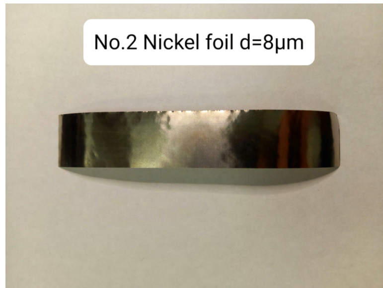
Figure 53 | Nonirradiated nickel foils marked as No.2 with thickness 8 \mu\text{m} and with fluence 8.31592 \cdot 10^{15} \text{ cm}^{-2} was used in degrader
