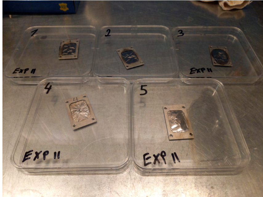
Figure 47 | Irradiated metal foils which was taken down from degrader with window holders
