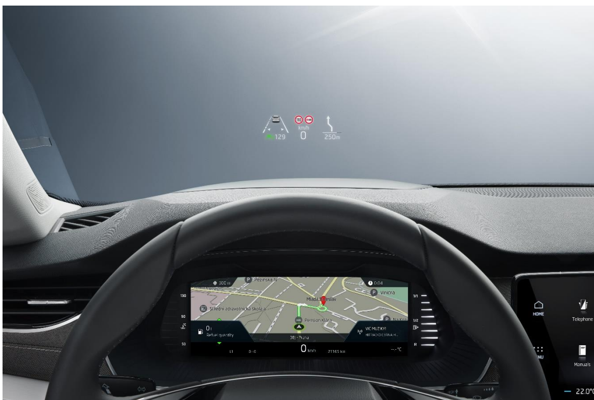
Obr. 6 Head-up display Škoda Auto Octavia
