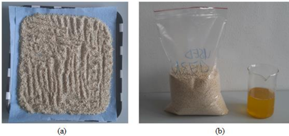
Figure 8. Sample of sesame seeds: (a) after test, (b) extracted oil in a beaker with the sample after test packed into a plastic bag.
