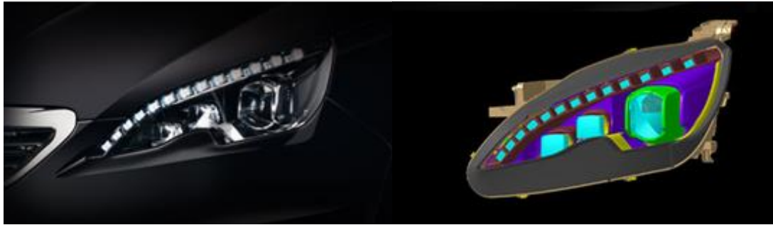
Figure 1.6.1.4 Example of a headlamp with a LED source a) in the final form, b) decomposed [2].
