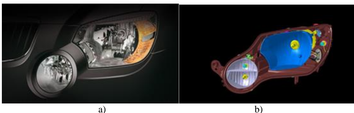
Figure 1.6.1.1 Example of a headlamp with a halogen bulb a) in the final form, b) decomposed [2].
