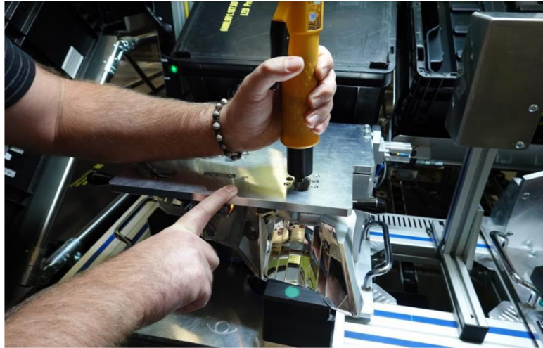
Figure 2.4.2.6 Assembly of the F-lux on the reflector with the screw using a direct pneumatic screwdriver.
