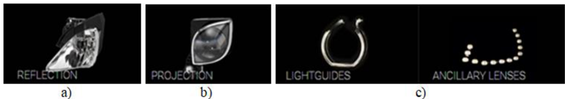
Figure 1.3.2.1 Examples of the optical systems a) reflection, b) projection and c) lightguides and ancillary lenses optical systems [2].
