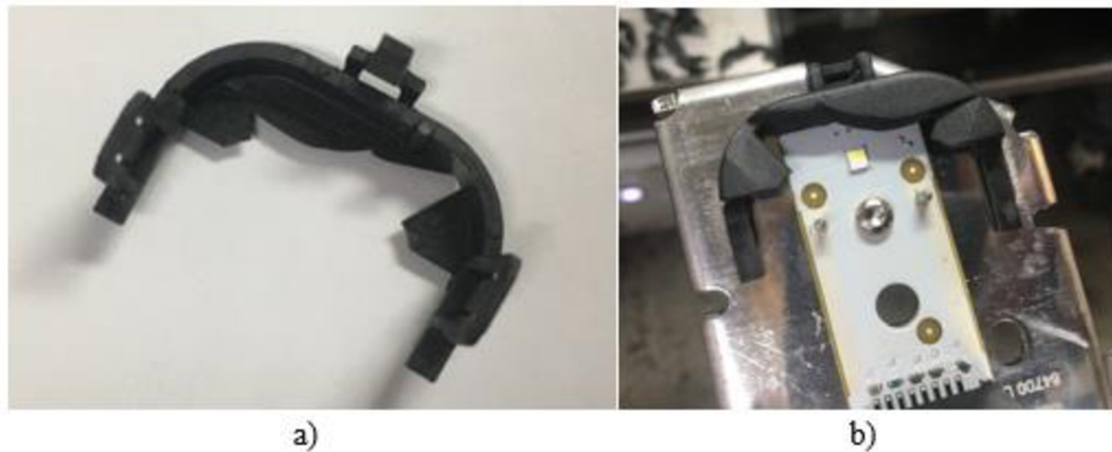
Figure 2.4.2.4 a) the plastic part to direct the light flow, b) the plastic part on the F-lux.
