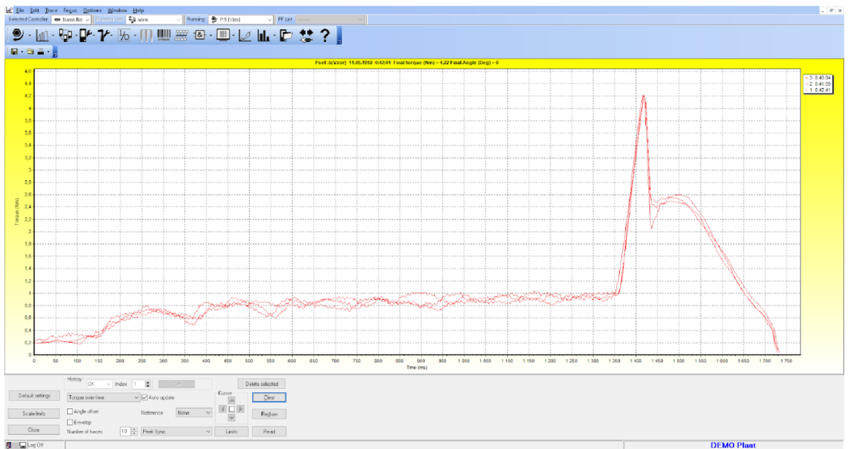
Figure 4.6.7.2 Example of the result of the measured torque using the tightening strategy of input in Atlas Copco.
