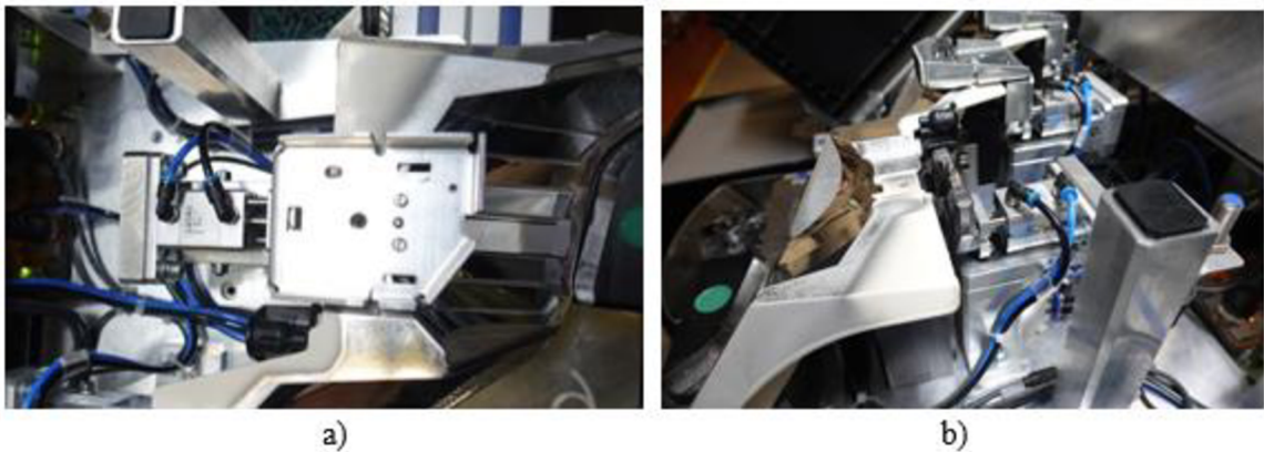
Figure 2.4.2.5 a) Detail on the pneumatic system, b) positioning of the F-lux.
