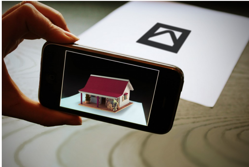
Figure 4.2: Augmented object position determination using QR-code Marker.[18]
