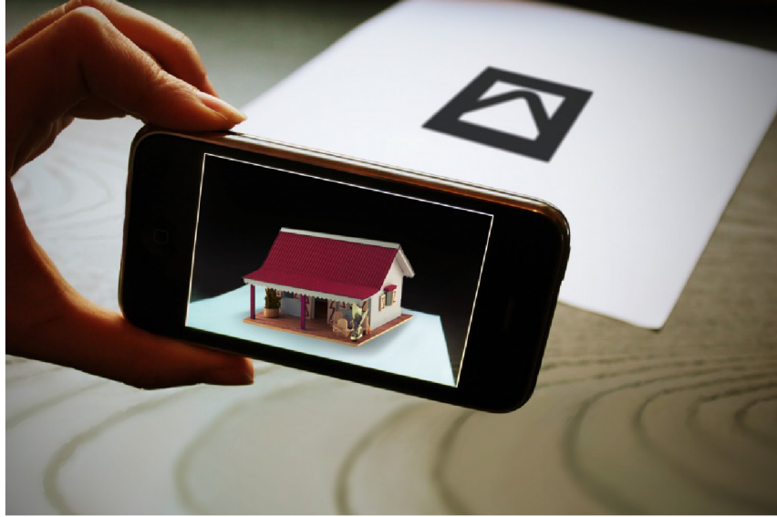
Figure 4.2: Augmented object position determination using QR-code Marker.[18]
