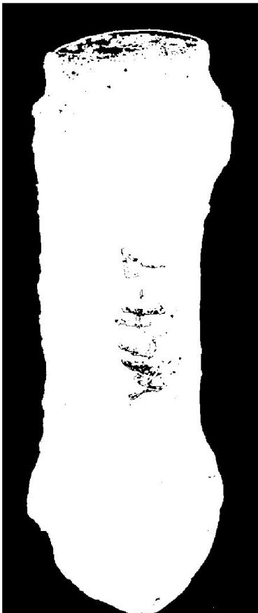
Figure A.1: HSV thresholding with Gaussian blur.
