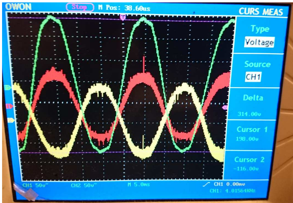
Figure 28: Voltage waveforms on the full-bridge output during initial testing. Generated voltage 112 V AC .
