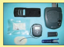
Fig. 2 CGMS: Sensor, monitor and connecting cable, con-station for data transfer, setter for sensor insertion, leader case for monitor
