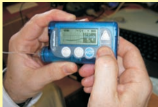
Fig. 2 Real-time glucose values displayed at screen of insulin pump Paradigm 722
