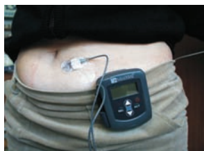
Fig. 1 CGMS Gold, Medtronic Minimed, Northridge, CA, USA; sensor connecting cable and monitor
