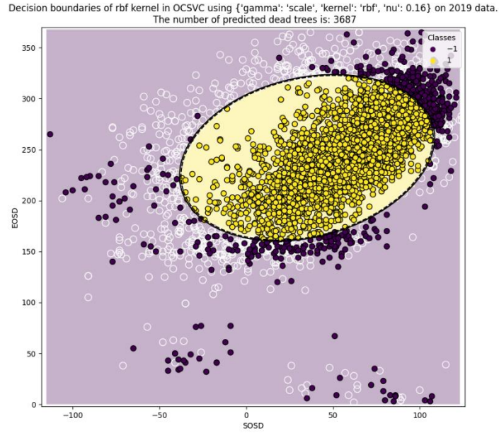
Figure A1. 4. Decision boundary for One-Class SVM for feature set of ['SOSD', 'EOSD'], using hyperparameters: {'gamma':'scale', 'kernel':'rbf', 'nu':0.16} on validation dataset #2 (2019). '1': dead tree prediction, '-1': outlier. Accuracy: 87.20 %
