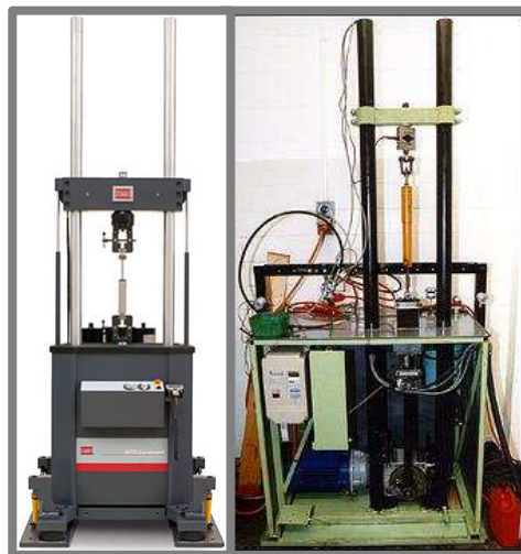
Obr. 2-14 Testery pre diagnostiku chovania tlmičov [15] [16]
