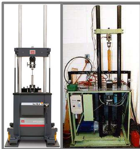
Obr. 2-14 Testery pre diagnostiku chovania tlmičov [15] [16]
