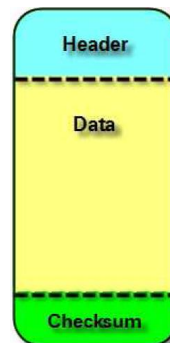
Figure 5. Structure of a Data Object
