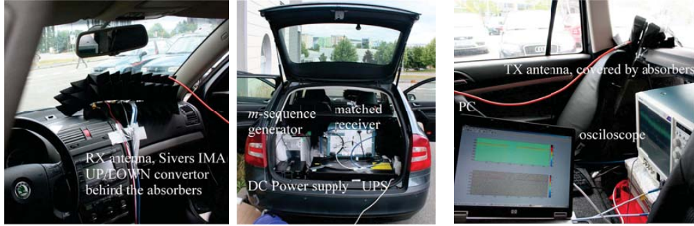
(a) The dashboard of the measurement vehicle. Behind the absorbers is the RX with both the up/down Siivers IMA converters and the LNA. (b) The trunk of the vehicle with the UPS power supply (good for around 1 hour of operation) and DC power supply for LNA and PA. (c) The back seat. The TX antenna is fastened on the rear quarter window using a suction cap. The PA and the is covered by absorbers.
