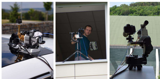
Fig. 5. From left to right: placement of TX antenna on the car roof, RX antenna on the gimbal head and on the motorized mount.
