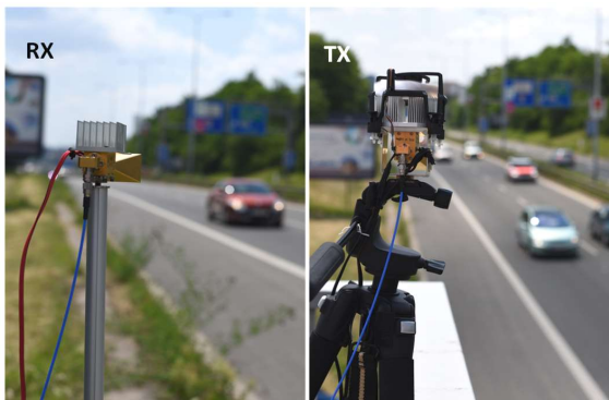
Fig. 10. Testing the channel sounder in “radar mode” on a highway.
