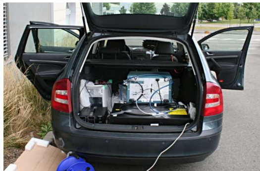
Fig. 3. Installation of the testbed into car Skoda Octavia 1.9 TDI.
