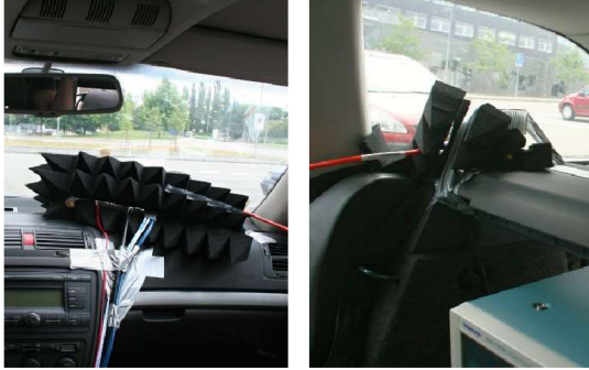
Fig. 4. Installation of the receiver (left) and transmitter (right).
