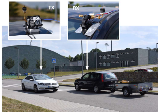
Fig. 7. Testing the channel sounder using two passing cars.
