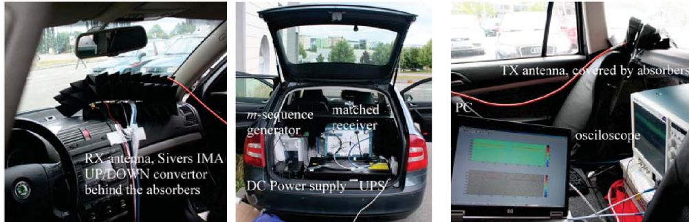
(a) The dashboard of the measurement vehicle. Behind the absorbers is the RX with both the up/down Siivers IMA converters and the LNA. (b) The trunk of the vehicle with the UPS power supply (good for around 1 hour of operation) and DC power supply for LNA and PA. (c) The back seat. The TX antenna is fastened on the rear quarter window using a suction cap. The PA and the is covered by absorbers.
