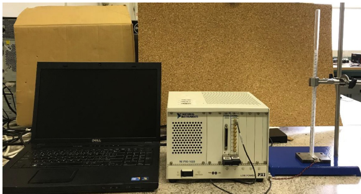
Figure 4-3 Ball Drop method experimental setup
