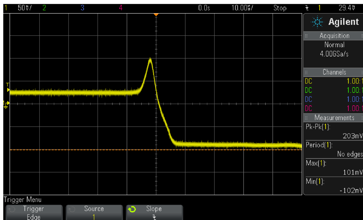
Figure 4-6 2mm diameter H pencil lead 20mm protruding length calibration signal obtained MSO-X-3054A oscilloscope
