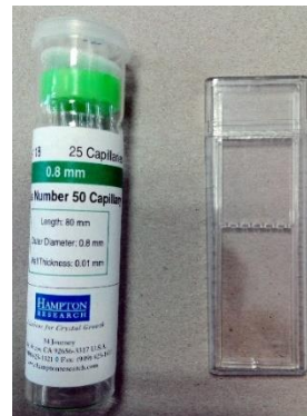
Figure 11. Capillary for free interface diffusion. (Picture created by the author)
