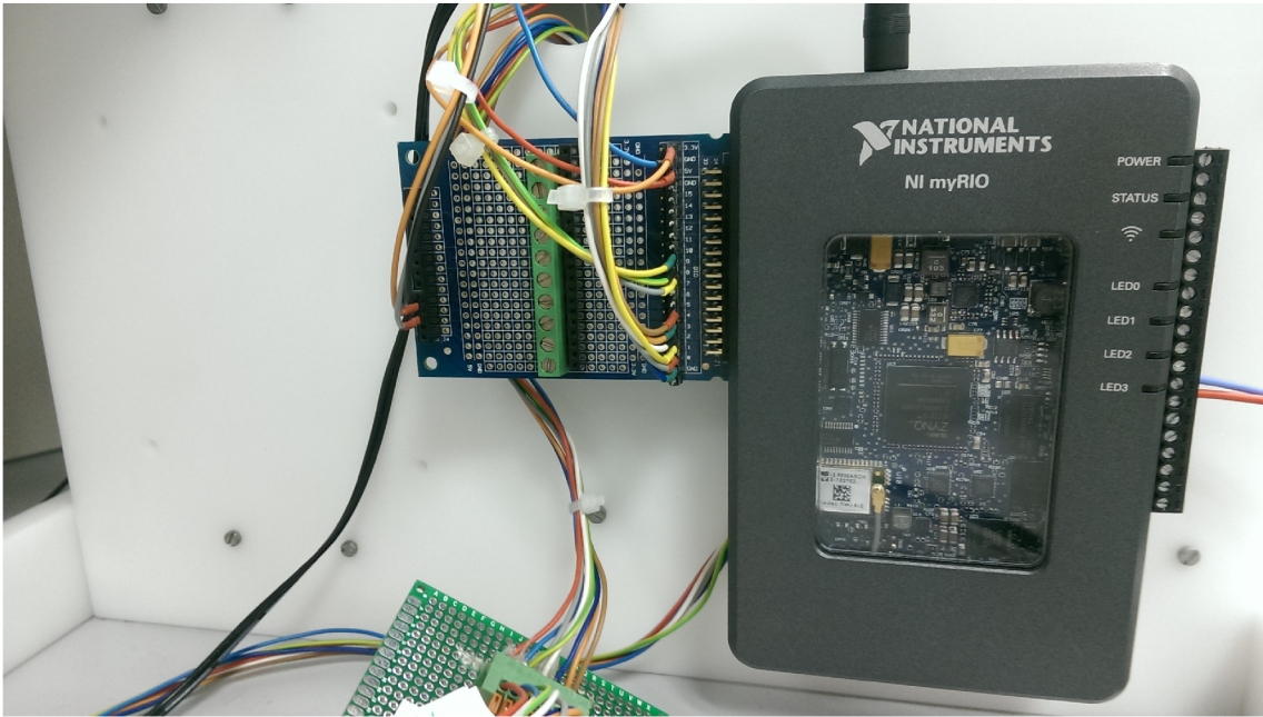
Figure 5.2: NI MyRIO with wired necessary connections.
