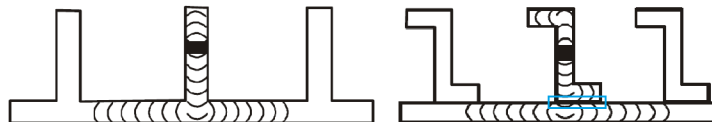
Figure 1.1: A comparison of integral and riveted structures: Physical barrier marked with blue colour [1].
