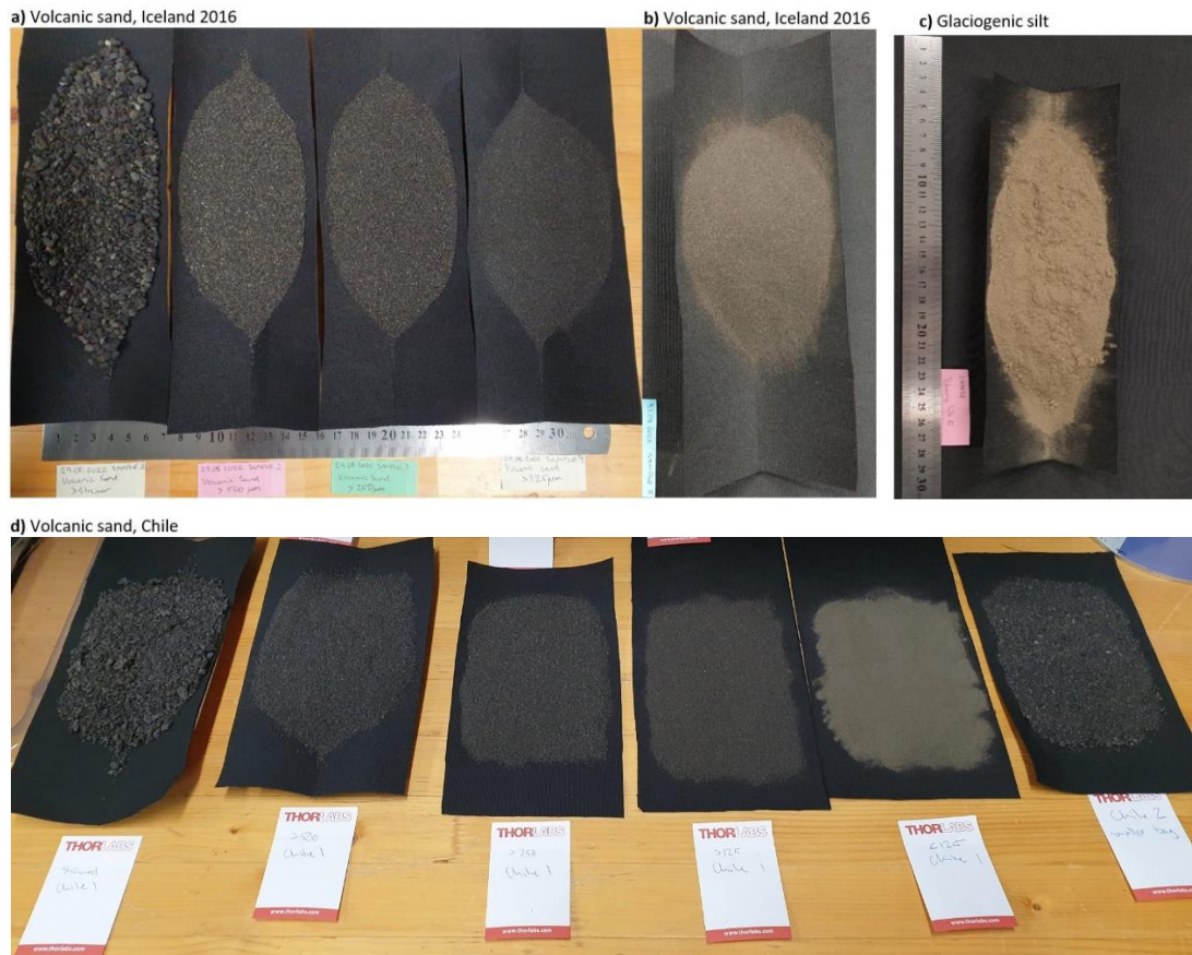
Figure 5. Samples in measurement trays. In a) Volcanic sand from Iceland 2016 can be seen as un-sieved, above 500 \mu\text{m} , above 250 \mu\text{m} and above 125 \mu\text{m} . In b) the same sample as in a) but sieved to under 125 \mu\text{m} . Picture c) shows glaciogenic silt sample. In d) from left to right Chile sample 1 un-sieved, above 500 \mu\text{m} , above 250 \mu\text{m} , above 125 \mu\text{m} , below 125 \mu\text{m} and lastly the Chile sample 2.
