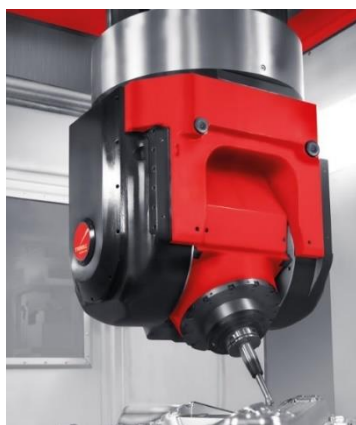
Obr. 9) Vidlicová hlava T30M, Trimill [11]
