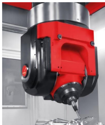
Obr. 9) Vidlicová hlava T30M, Trimill [11]
