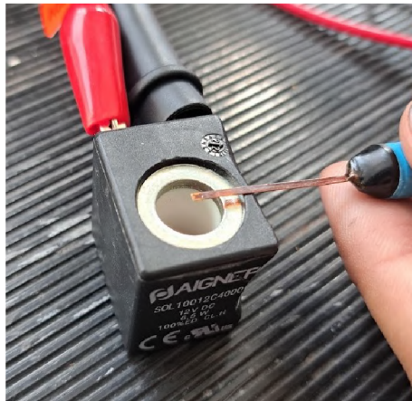
Figure 6.2.3: Coil measurement with Hall probe
