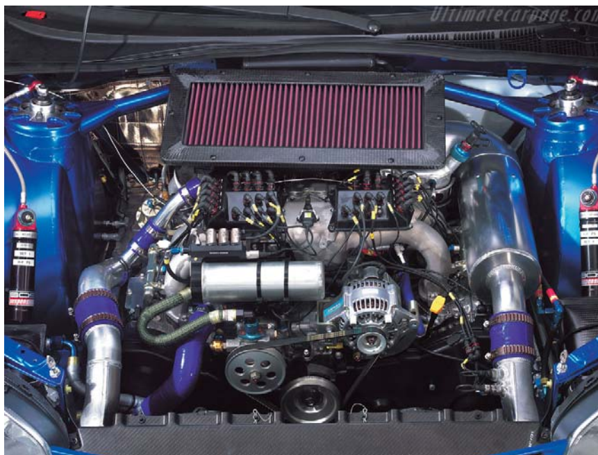
Obr.19 Subaru Impreza WRC s motorem Boxer o obsahu 2000ccm [40]
