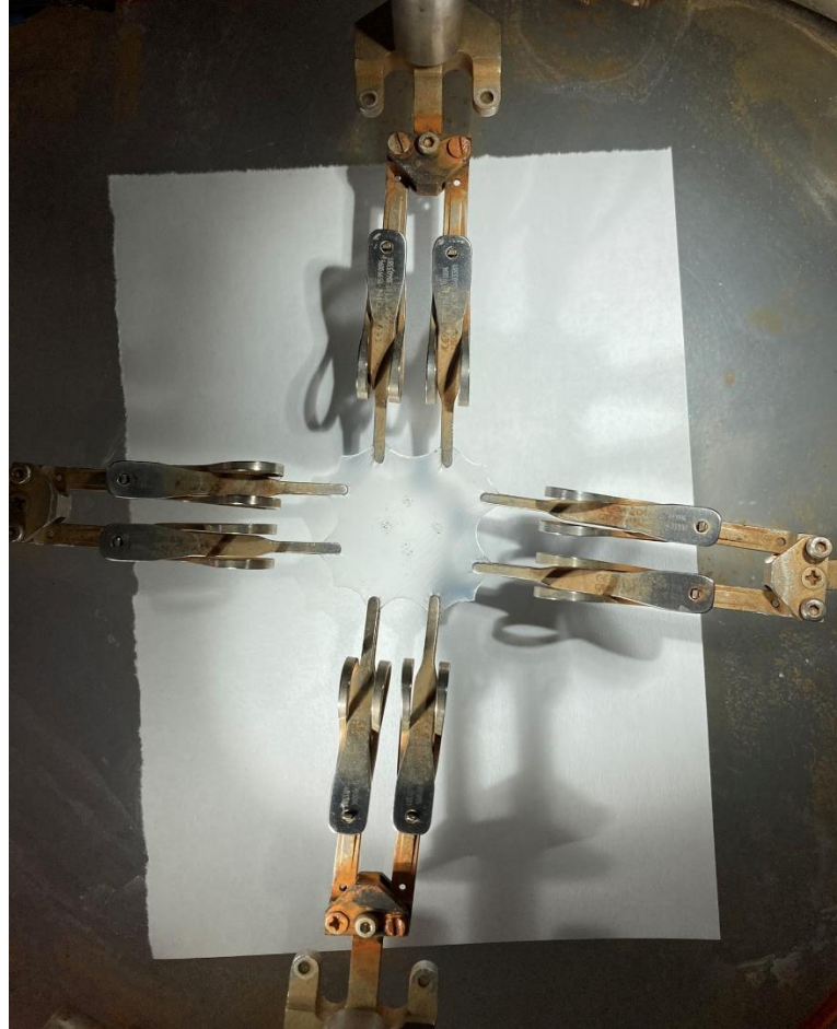
Figure 22: The testing device used to determine the Young's moduli of silicone compounds used in the thesis.
