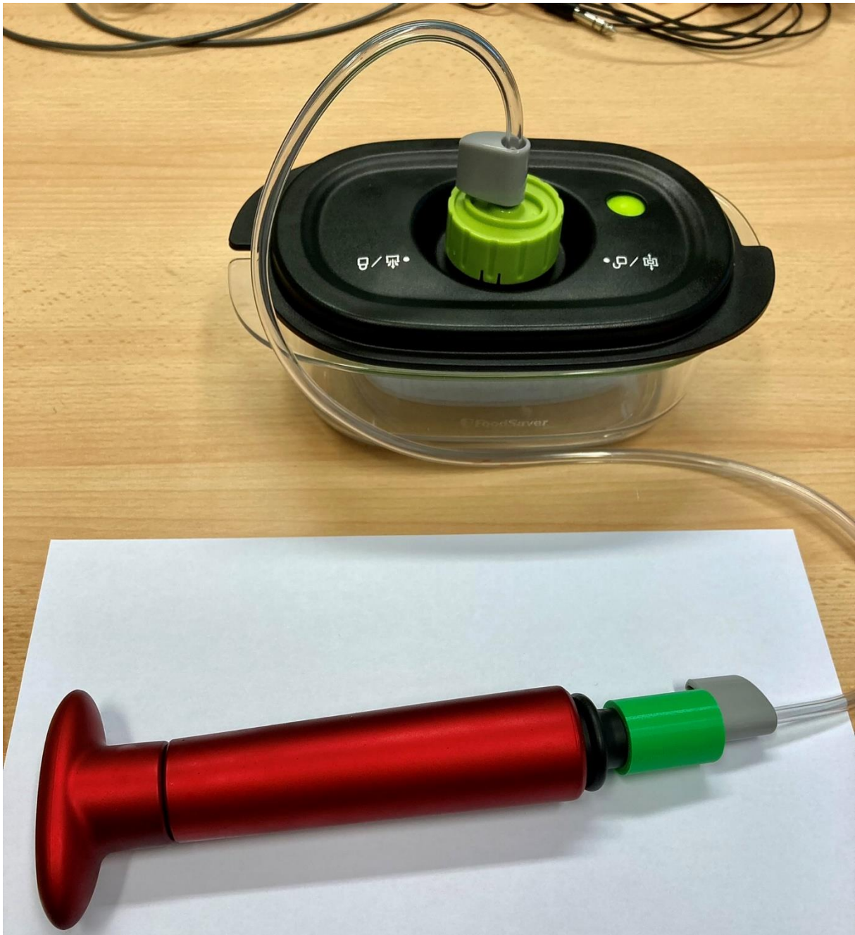
Figure 24: Vacuum chamber used to remove air from the silicone compounds.
