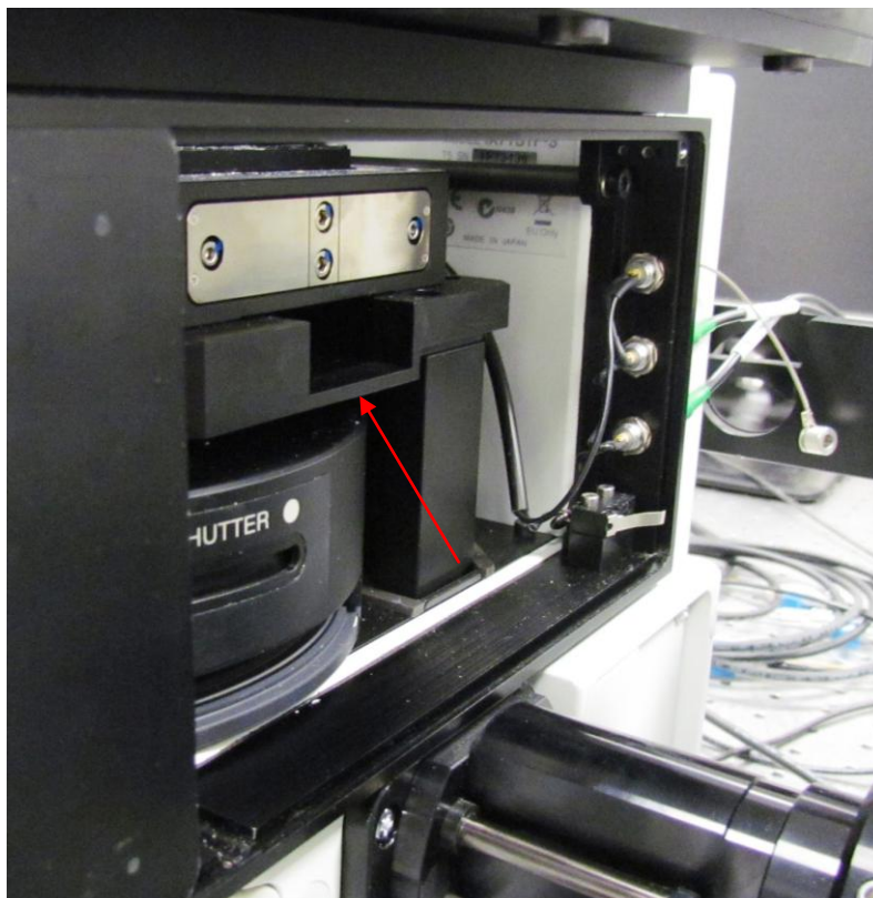
Fig. 12: The microscope body with description where put the Nomarski prism (red arrow).
