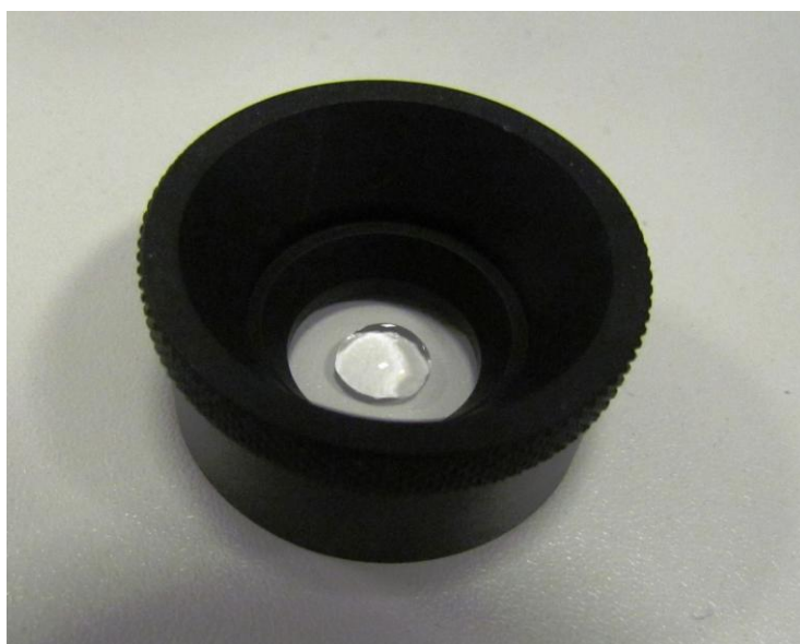
Fig. 8: The sample holder with glass slide and drop of sample.
