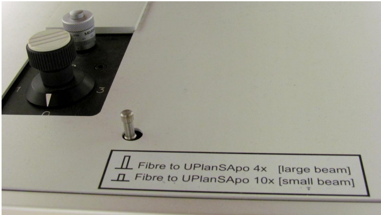
Fig. 5: The position of button in the small beam regime.
