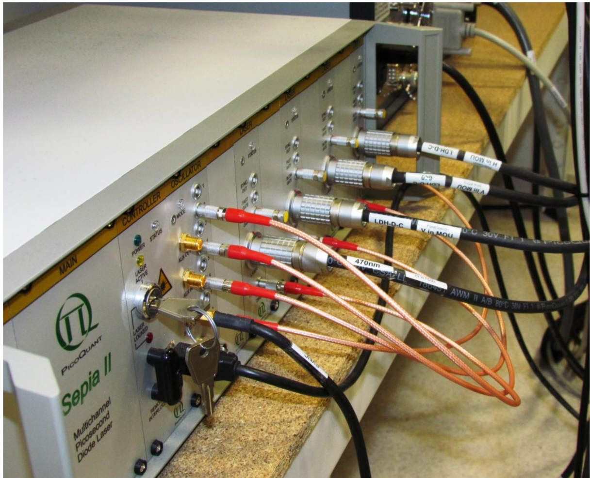
Fig. 4: The connections of laser heads to multichannel diode laser unit.
