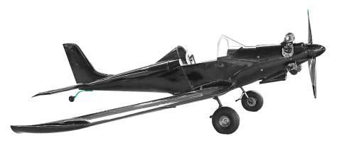
Figure 7.2: Tail gear spring (in green): Merlin Sportster. Courtesy of TechProAviation, s.r.o.
