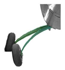
Figure 2.16: Composed picture of main landing gear during drop test. Un-deformed and maximum deformation. Courtesy of TechProAviation, s.r.o.
