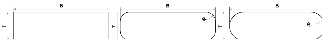
Figure 4.25: Rectangular cross-section without radius, with mid-size radius and with rounded edges (maximum radius).
