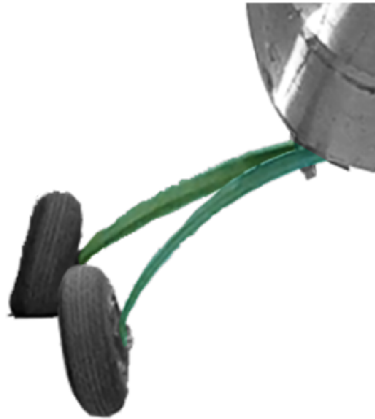
Figure 2.16: Composed picture of main landing gear during drop test. Un-deformed and maximum deformation. Courtesy of TechProAviation, s.r.o.
