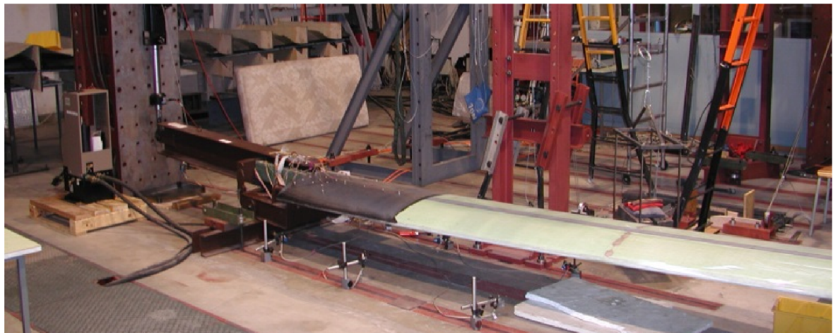
Figure 5.1: Layout of X06 wing segment fatigue test. Archive of IAE.
