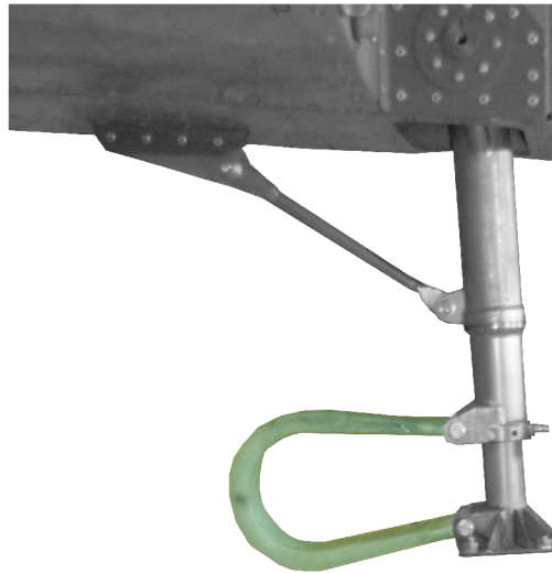
Figure 7.1: Nose gear spring (in green) on Merlin 105 airplane. Courtesy of TechProAviation, s.r.o.
