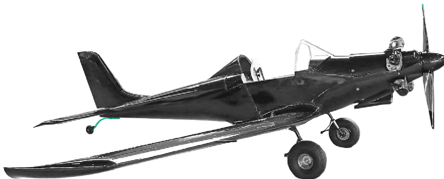
Figure 7.2: Tail gear spring (in green): Merlin Sportster. Courtesy of TechProAviation, s.r.o.
