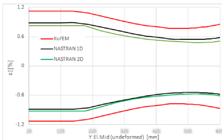
Figure 5.20: Comparison of \epsilon_1 strains obtained from KuFEM and NASTRAN.
