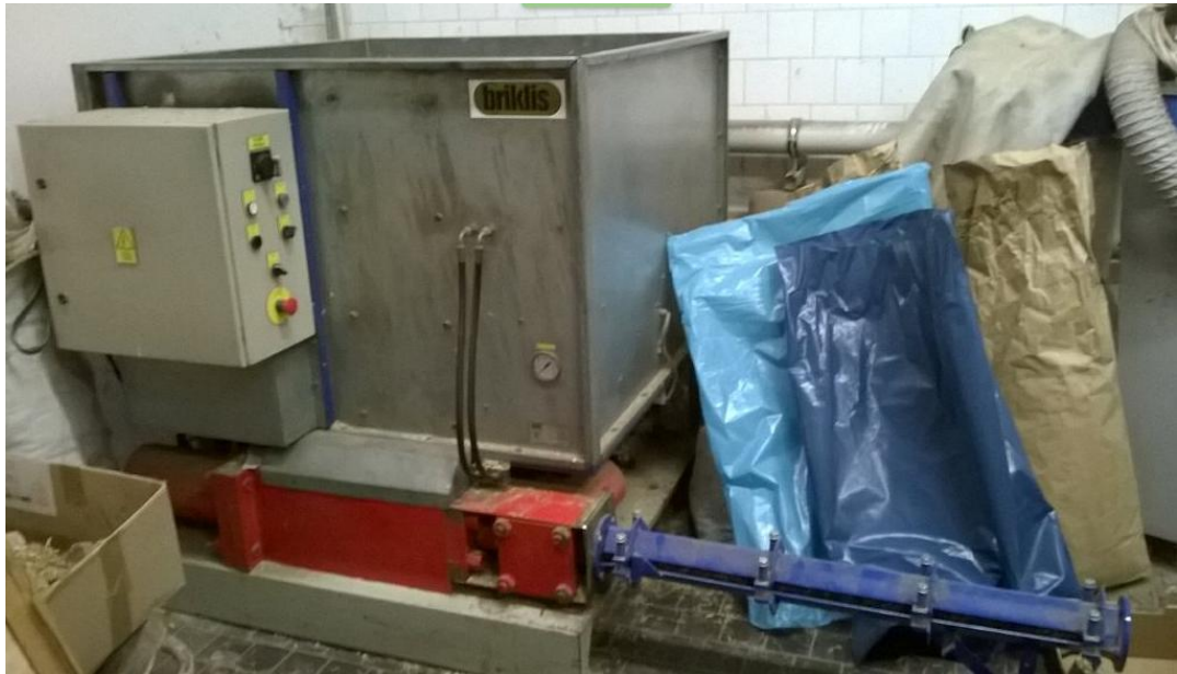
Figure 7: Hydraulic piston briquetting press BrikStar CS 50 at RIAE
