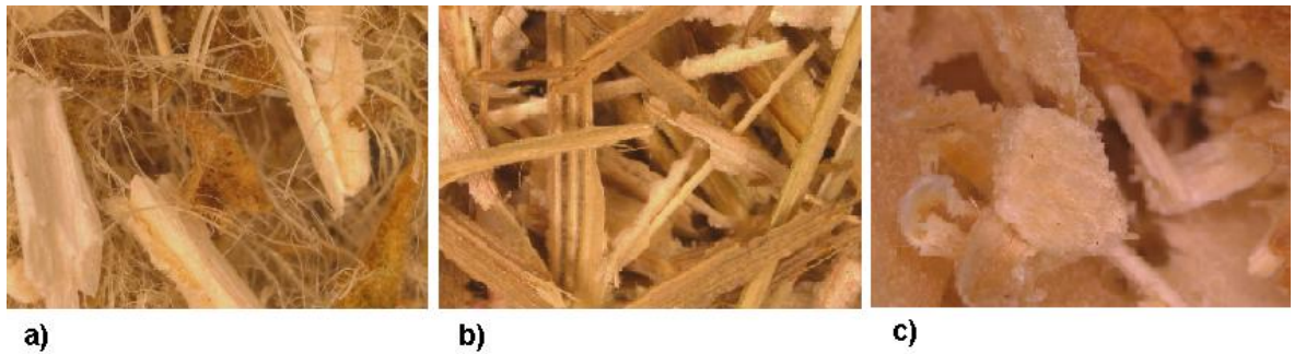
Figure 21: Undensified materials before briquetting
