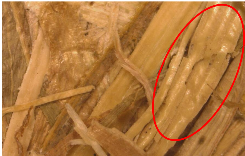
Figure 22: Typical glassy coating of natural binders on biomass particles
