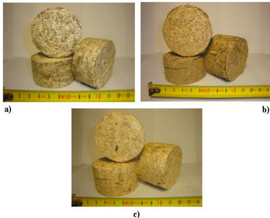
Figure 19: Produced briquettes made of different biomass sources
