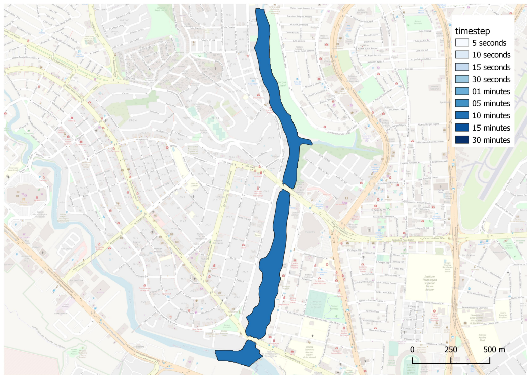
Figure E.21: Maximum water surface elevation output for a upstream boundary condition of ten-years return period hydrograph, main channel roughness = 0.066 and flood plain roughness = 0.144, and time step = 10 minutes.
