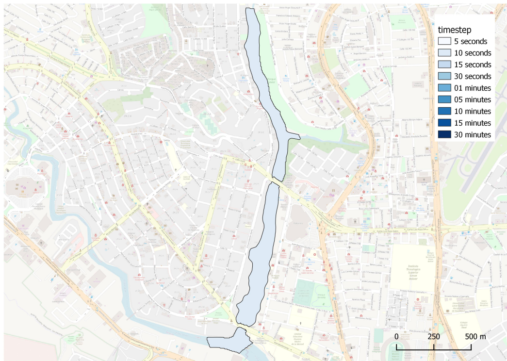
Figure E.17: Maximum water surface elevation output for a upstream boundary condition of ten-years return period hydrograph, main channel roughness = 0.066 and flood plain roughness = 0.144, and time step = 10 seconds.
