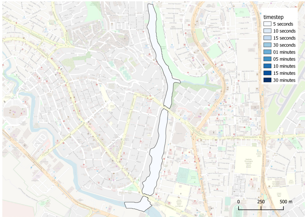
Figure E.16: Maximum water surface elevation output for a upstream boundary condition of ten-years return period hydrograph, main channel roughness = 0.066 and flood plain roughness = 0.144, and time step = 5 seconds.
