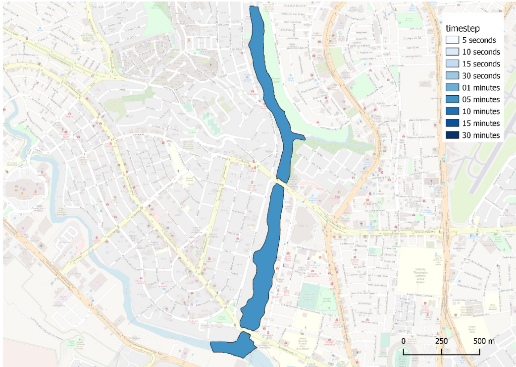
Figure E.20: Maximum water surface elevation output for a upstream boundary condition of ten-years return period hydrograph, main channel roughness = 0.066 and flood plain roughness = 0.144, and time step = 5 minutes.
