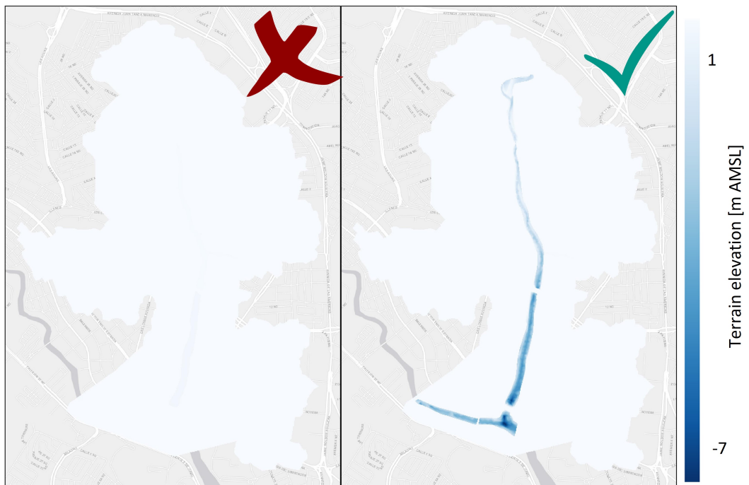
Figure 2.5: Comparison between (left) initial DEM of 5m \times 5m resolution - orthophoto and (right) updated DEM - measured bathymetry
