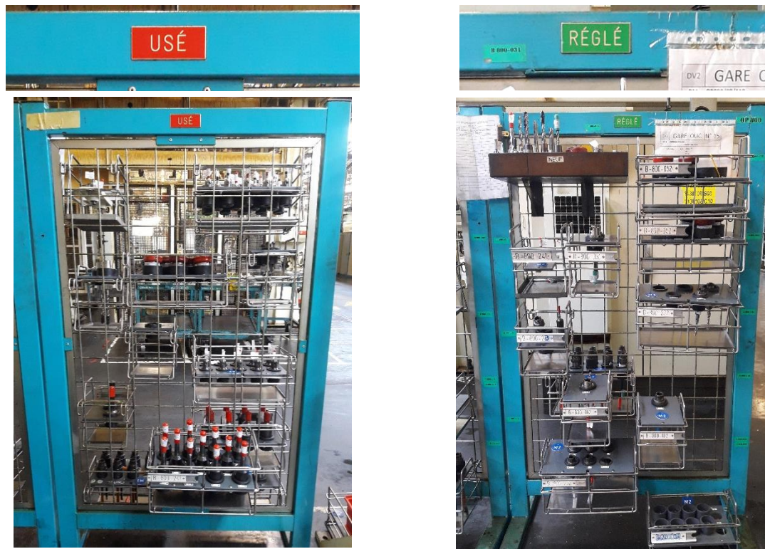
Figure 5.1.10.1 - Worn cutting tools (on the left) , pre-set cutting tools (on the right)
