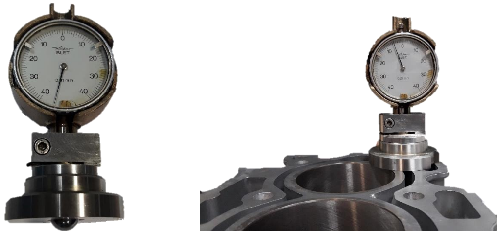
Figure 5.2.2.7 measurement of dimensions by the dial gauge with the special probe, the dial indicator assembled with the holder (on the left), the spring and the half-spherical probe, the dial indicator mounted on the reference bore (on the right)
