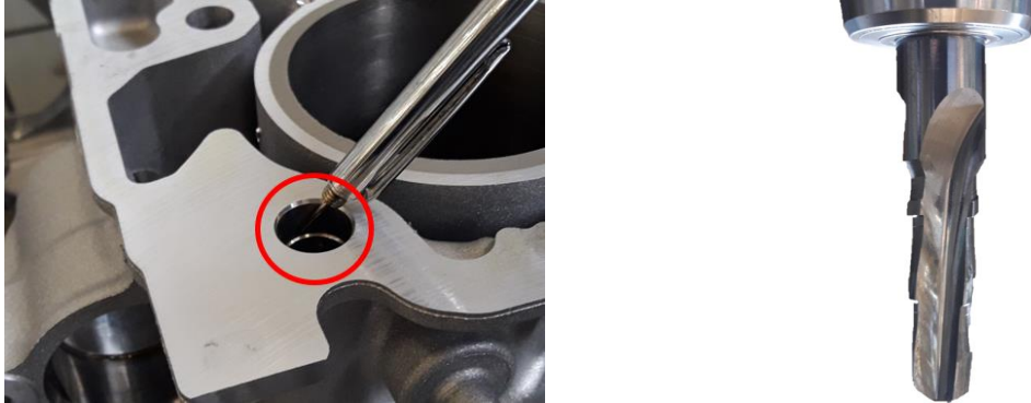
Figure 5.2.2.6 The reference bore, position of the bore on the cylinder head plane (on the left), the stepped reamer machining the reference hole at OP10 (on the right)
