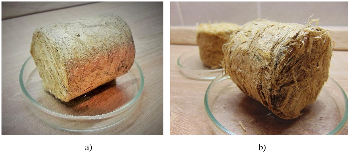
Figure 25: Investigated bio-briquette samples: a) before DU test, b) after DU test
