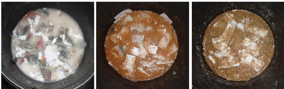
Figure 20: Feedstock materials prepared for compression: a) waste paper, b) waste paper + sawdust (1:1), c) waste paper + rice husk (1:1)
