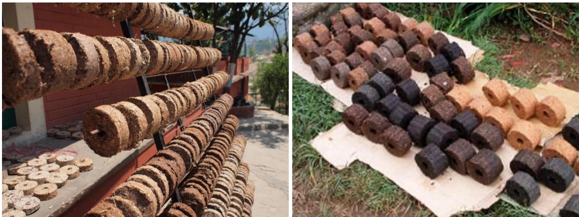
Figure 4: Examples of various bio-briquette samples produced by low-pressure briquetting presses (Source: Engineeringforchange.org; Legacyfound.org).
