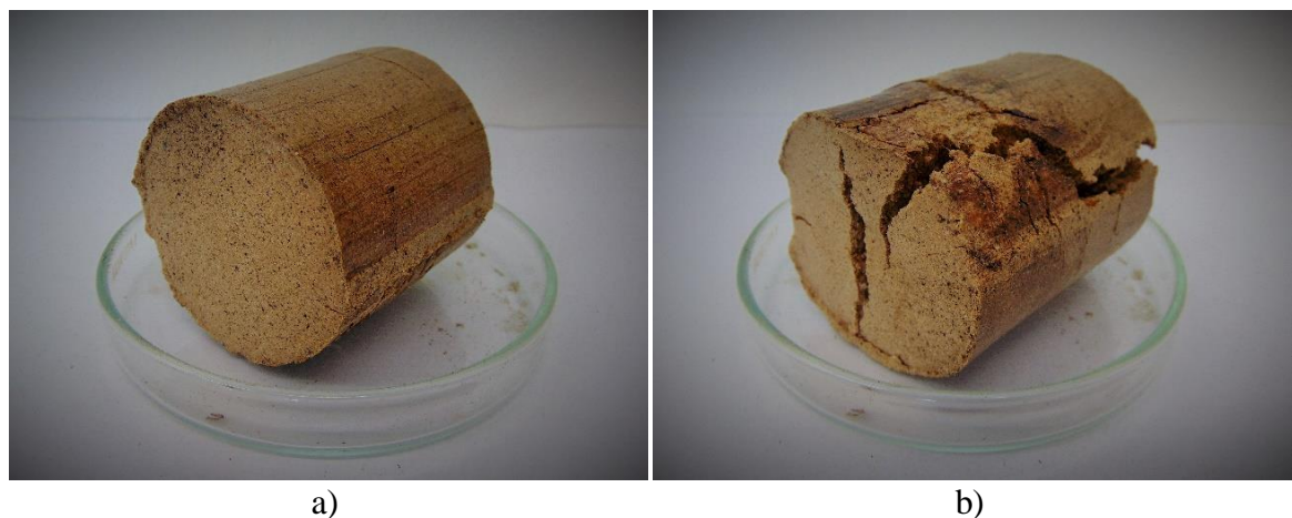
Figure 24: Investigated bio-briquette samples: a) before RF test, b) after RF test
