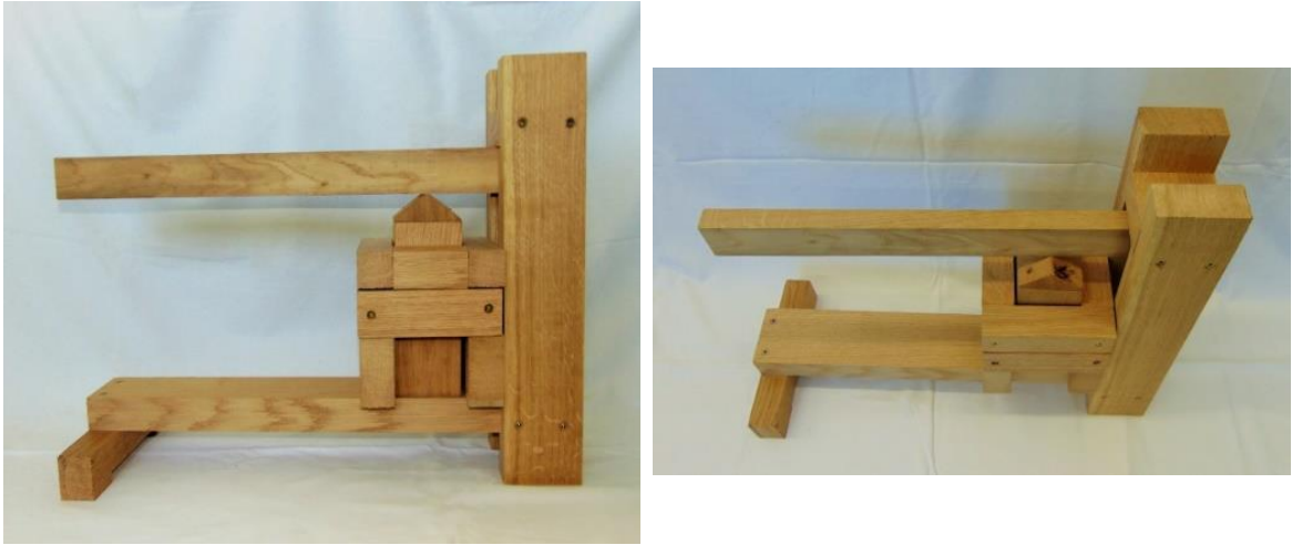
Figure 32: Developed manual low-pressure briquetting press from wood components.
