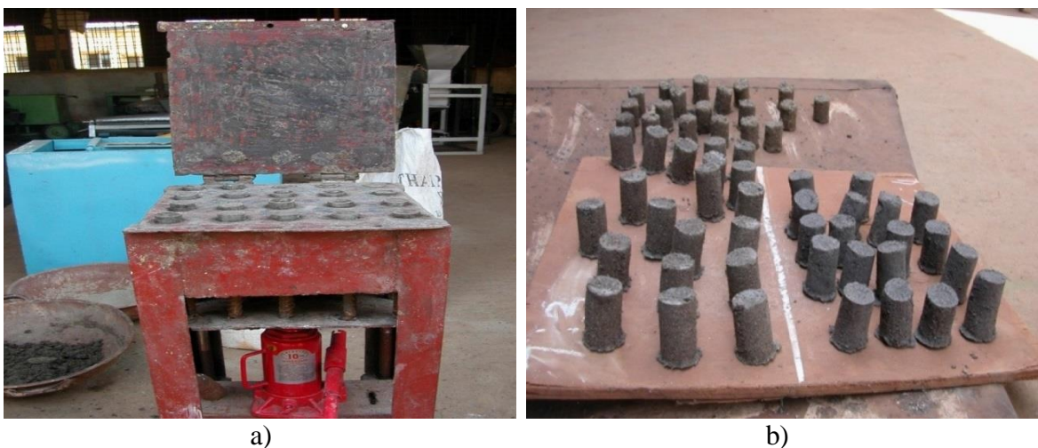
Figure 6: a) Low-pressure moulding machine, b) produced bio-briquette samples [128]
