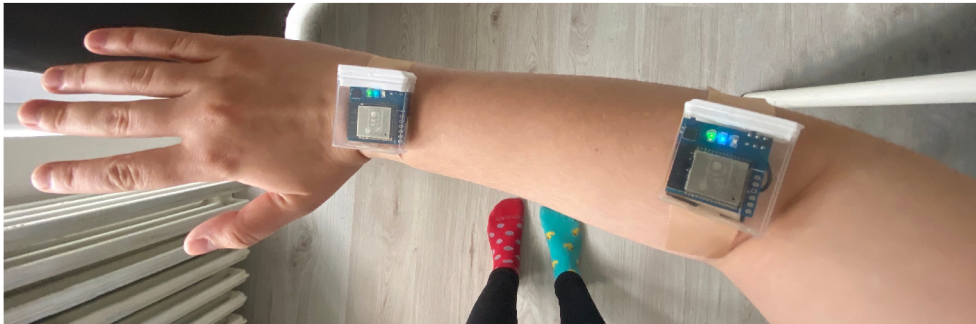
Figure 7.4: Two mo-cap bands positioned on a subject’s arm. The blue LEDs indicate an active Wi-Fi connection, the green ESP-NOW synchronization.
