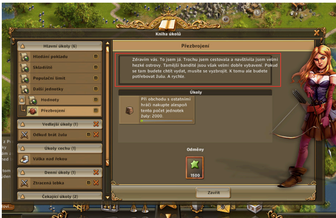
Figure 10: Provided screenshot shows a cut-off (marked red) of an objective (quest) in a browser game The Settlers Online . Such issue can prevent the player from proceeding in the game as it is unclear what the task of this quest is. A suitable fix for this problem is either to provide a wider box for the whole line to fit or make the cut-off text appear under the first line by making a line break.
