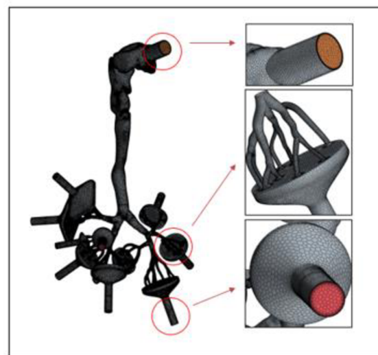
Figure 17: polyhedral mesh contour of the model geometry of human lungs
