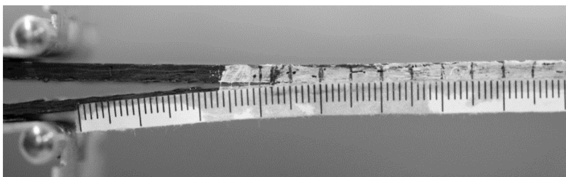
Figure 30: DCB, CNTs specimen (poor material quality), initial crack length
