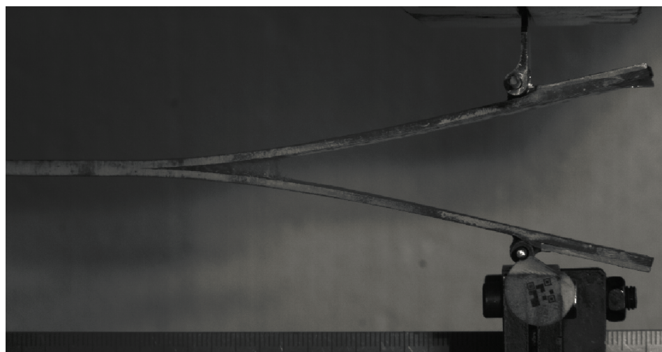
Figure 41: DCB-BUT, Test setup – end crack length
