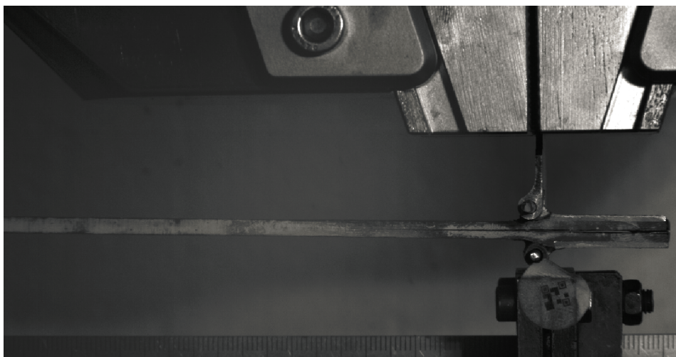
Figure 40: DCB-BUT, Test setup – initial crack length
