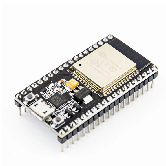
Figure 1.3: ESP32 development board Source: https://rpishop.cz
