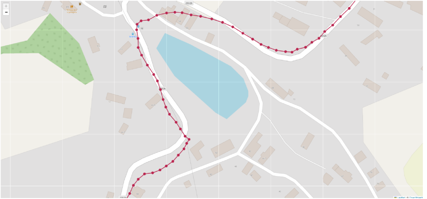
Figure A.6: The amount of captured detail with a sampling rate of 1s
