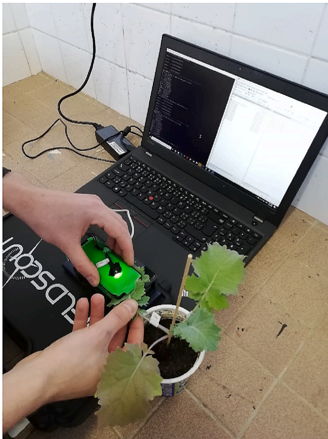
Fig. 4. The proposed Rasp2SPAD prototype in the evaluation procedure on the winter rapeseed.
