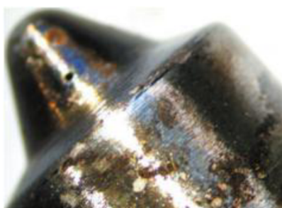
Obr. 24: Koroze na hrotu trysky [12]
