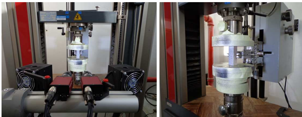
Fig. 3.2.1-1: The experimental setup for the compression test parallel to the grain (Paper I)
