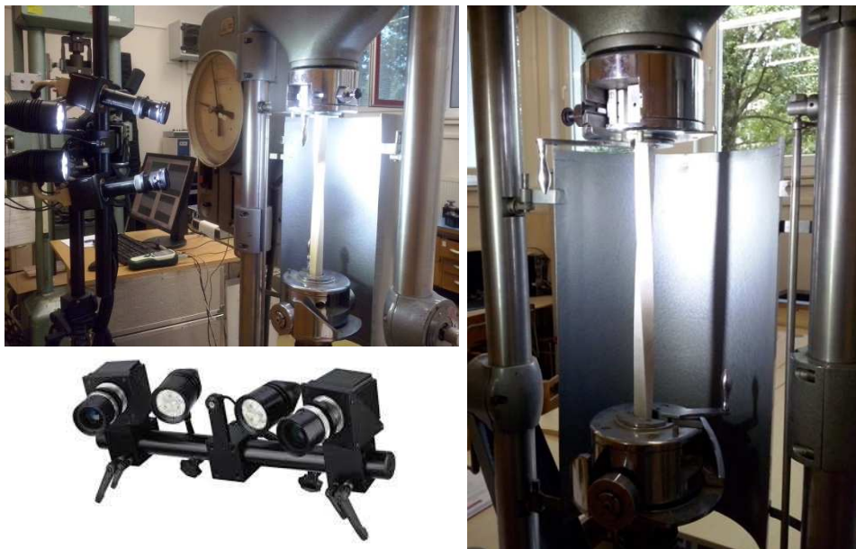
Fig. 3.2.1-3: The experimental setup for the torsion test around longitudinal axis (Paper III)
