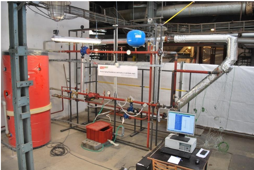
Figure 4.2 – Experimental setup of tubular heat exchanger.
