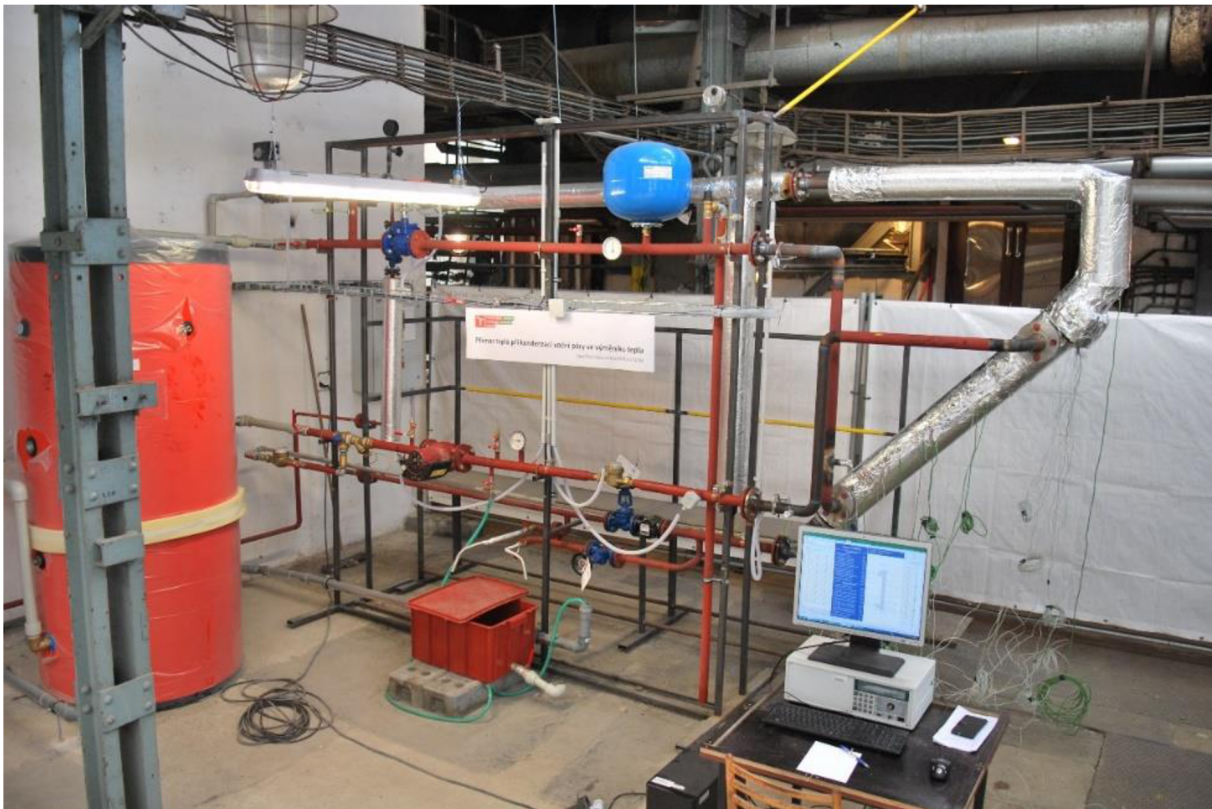
Figure 4.2 – Experimental setup of tubular heat exchanger.
