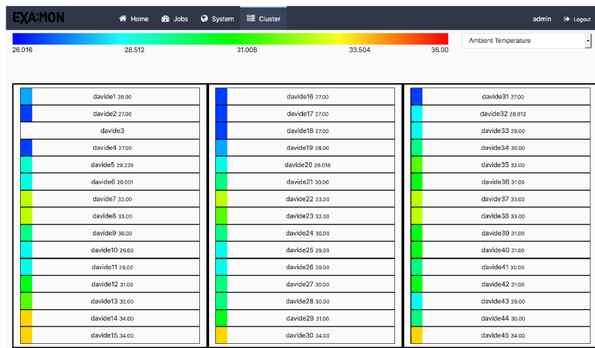
Figure 5.9: The 2D HTML generated model of D.A.V.I.D.E. supercomputer supplied with data via WebSockets.
